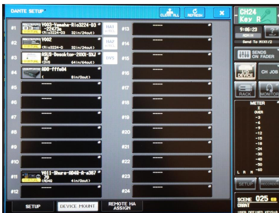
Figure 6 – The unit is now mounted on slot #4 and reported as 8in/0out. The UNSUPPORTED label simply means it is not a Yamaha I/O device.
