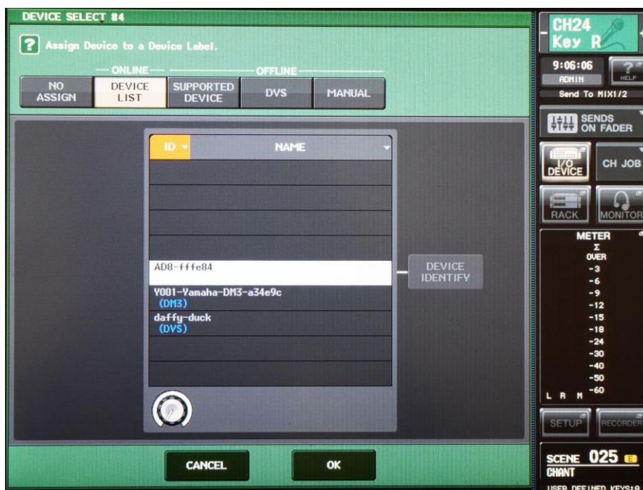
Figure 5 – In the DEVICE SELECT window, press DEVICE LIST , select AD8-xxxxxx and confirm with OK .
