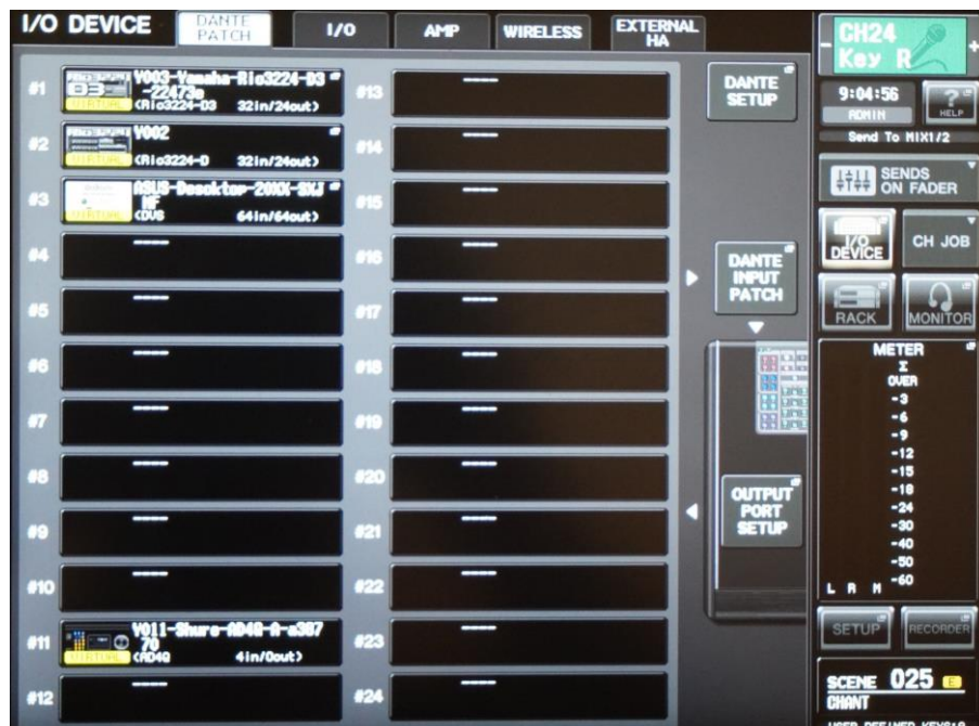
Figure 2 – The I/O DEVICE screen opens on the DANTE PATCH tab, which lists the devices already mounted (#1 to #24).
