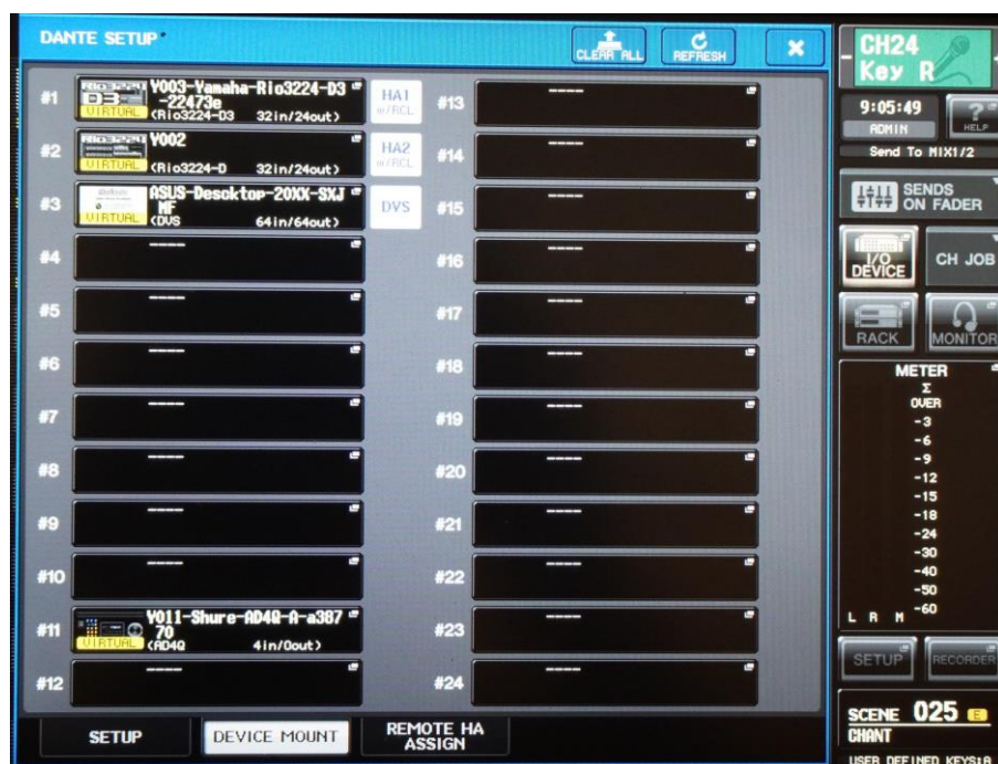
Figure 4 – Select the DEVICE MOUNT tab, then press a free slot – here #4.
