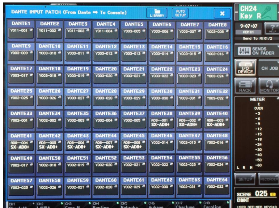
Figure 7 – DANTE INPUT PATCH. Ports DANTE38 to DANTE45 carry the eight SX-AD8+ channels (AD8--001 to AD8--008).
