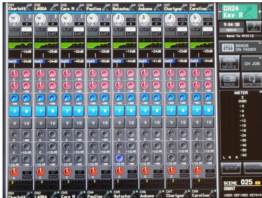
Figure 1 – From any screen, press the I/O DEVICE button on the right-hand side of the display.
