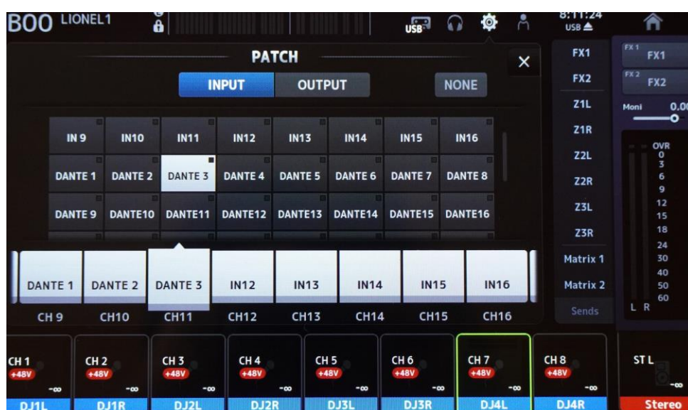
Figure 3 – Setup → Patch, INPUT tab. The lower row shows the console channels; the grid above lists the available sources. Here DANTE 1, DANTE 2 and DANTE 3 have been assigned to CH9, CH10 and CH11.
